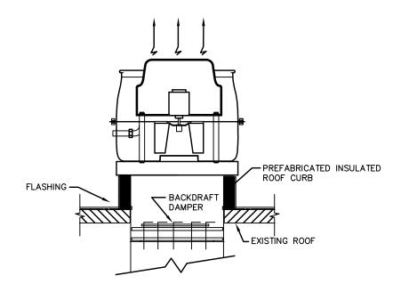
UPBLAST GENERAL EXHAUST FAN AND CURB DETAIL
