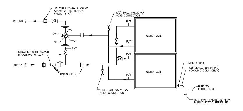
STACKED WATER/FLUID COIL SINGLE PIPING DETAIL W/ 3-WAY CONTROL VALVE
