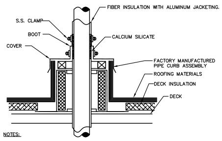
1. PROVIDE ROOFING PENETRATION APPROVED AND INSTALLED BY U.S. ROOFING. COORDINATE REQUIREMENTS AND INCORPORATE INTO BID.
