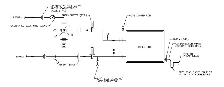
SINGLE 3-WAY WATER/ FLUID COIL PIPING DETAIL W/ 3-WAY CONTROL VALVE
