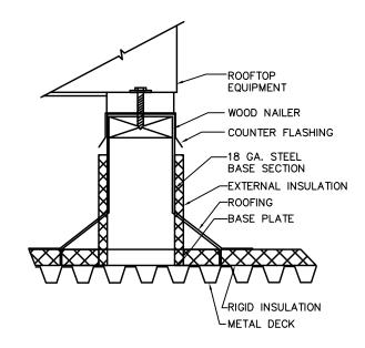
NON- CANTED EQUIPMENT ROOF SUPPORT DETAIL SCALE: NTS
