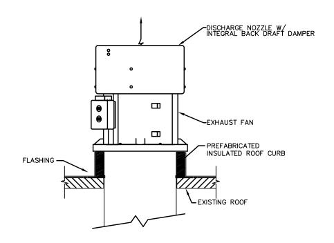
MIXED FLOW UPBLAST EXHAUST FAN AND CURB DETAIL
